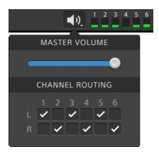
Drag the Master Volume fader to increase or decrease audio levels. During preview, the meters allow you to monitor the level of each audio channel.
