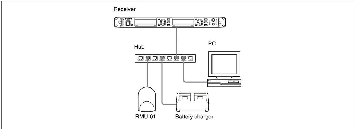
Use straight LAN cables to connect the receivers, RMU-01, battery chargers, and computer via a hub. When the network connection is correctly made, the LED on the LAN connector area at the rear of the receiver lights up green.
